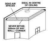
Place the alarm on the ceiling/wall and mark the screw holes. Drill with a suitable drill bit, insert the screw plugs and screw the alarm into position. Simply connect the battery on the alarm and slide into position on the mounting plate.
